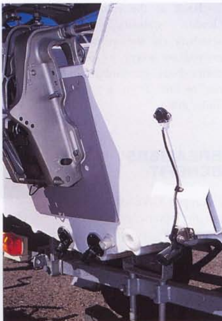
Quinnie doesn't muck around! Big drain plugs, live tank plumbing and a factory-fitted transducer plate are standard.
